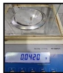
Fig (4): Measuring body weights of each stage of larvae using a sensitive electrical balance with a sensitivity of nearest 1 milligram (mg).
